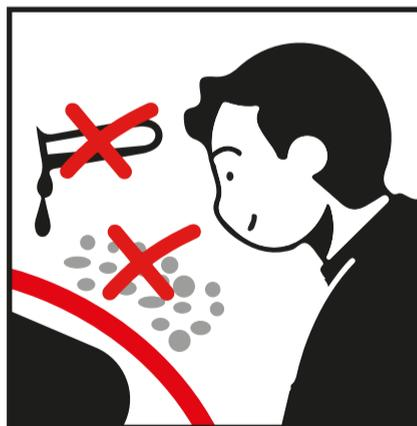
Ensure that the parts of the products directly in contact with the ground are never covered by the ground and do not come into contact with chemical or abrasive substances (lime, tuff stone, fertilisers, herbicides, etc.).
