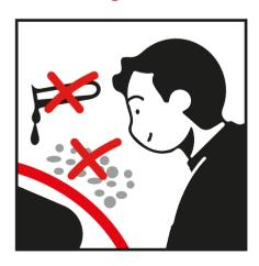
Ensure that the parts of the products directly in contact with the ground are never covered by the ground and do not come into contact with chemical or abrasive substances (lime, tuff stone, fertilisers, herbicides, etc.).
