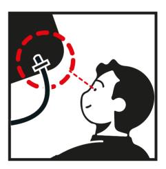
Check the fastening and integrity of all cable glands and power cables.
